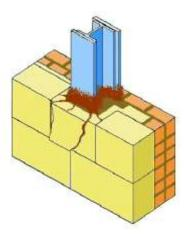
When metal corrodes it expands by seven to ten times the volume of the original metal. In this way, relatively low levels of corrosion can create large tensile forces within the masonry, causing cracking and displacement of the cladding, without structurally significant section-loss. The parallel cracking at beam and column locations is often referred to as Regent Street Disease.
